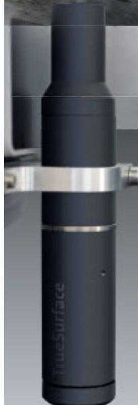
**WITec's new TrueSurface™ Microscopy** allows confocal Raman imaging guided by surface topography. The result is an image revealing chemical properties at the surface of the sample, even if it is rough or inclined.
